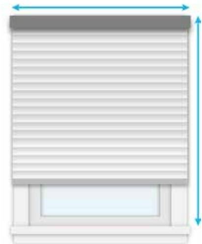
**1.** Measure the distance from the outermost points you would like the blind to cover. To minimize light leakage the blind should overlap the window opening by at least 1-1/2" on each side (3" total width).
