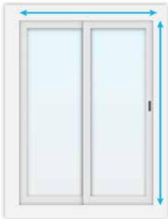
**1.** Measure the distance from the outermost points you would like the blind to cover. To minimize light leakage and ensure privacy the blind should overlap the window opening by 4" on each side for a total of 8" on entire width.
