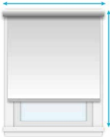
**Tip-to-tip:** Measure the distance from the outer most points you would like the headrail to extend. Depending on the product, the fabric width will be up to 1-3/8" narrower than the tip-to-tip measurement provided. The exact amount of fabric deduct can be obtained by contacting customer service. To minimize light leakage add 1-3/8" for fabric deductions, then add additional inches for desired overlap.
