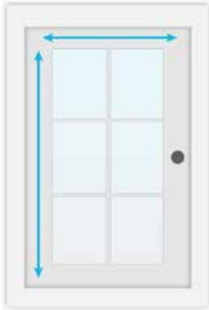
**1.** Start your measurement a minimum of 2" above the glass (3" recommended) and measure down 2" below the glass. This will provide enough room to mount installation brackets at the top and hold down brackets at the bottom. Extra height above your window should be allowed if you prefer the blind or shade to stack up above the glass and provide a less obstructed view. Call our customer service team for specific stack specifications **1-888-767-7856**.
